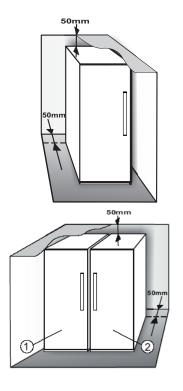
We recommended installing two appliances together using the linking-kit ③ (as shown on the drawing). You can buy it in Service.
