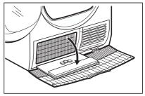
5. If necessary, remove the fluff from the condenser and its compartment. You can use a wet cloth and/or a vacuum cleaner with a brush attachment.
