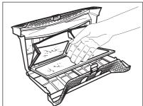
**4.** If necessary, clean the filter with a vacuum cleaner. Close the filter.
