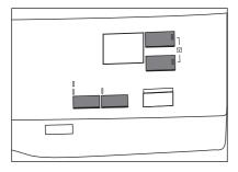
To activate or deactivate an option touch the relevant button or a two button combination.
