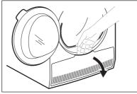
Turn the lever to unlock the condenser lid.
