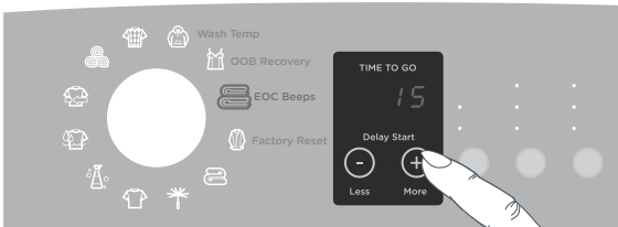
Fig.27 Modifying the number of beeps to signal the end of the cycle
