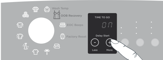
Fig.26 Changing the out of balance recovery routine
