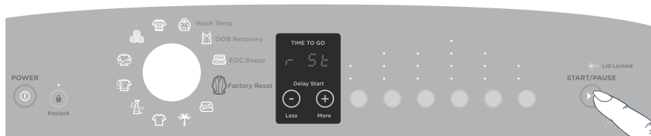
Fig.28 Changing the washer settings back to the factory default
