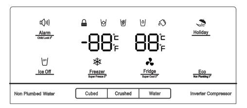
When the appliance is powered on for the first time, the backlighting of the icons on the display panel starts working. If no buttons have been touched and the doors are closed, the backlighting will turn off after 60 seconds.
