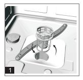
Step 1: contrarotate the Coarse filter , then lift it up:
