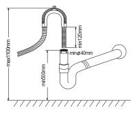
Fit the drainage hose of your machine to the drainage pipe without bending.
