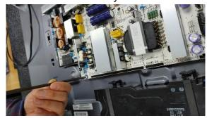
OLED Panel (together with their casing) is only left after all other parts like electronic units have been removed.
