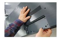
Once removed, this will expose the accessible electronic units (PCBs) which can now be easily removed with hand and screw driver.
