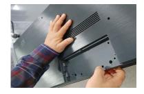
Once removed, this will expose the accessible electronic units (PCBs) which can now be easily removed with hand and screw driver.
