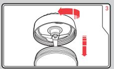
Ensure the Safety Seal (7) is fitted correctly. Attach the Blade Lid (3) to the Beaker. Screw to fix into place securely.
