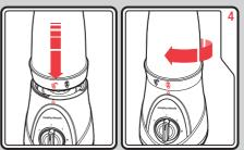
Attach the Blade Lid to the Main Unit (4). Align the open padlock and arrow and twist to lock into place.
