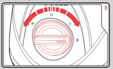
Plug into the mains. Turn the Control Knob (5) to the desired speed High (II), Low (I), or Pulse (P). Your Blend Express will begin to blend.
