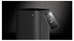
Pair Bluetooth® devices easily with one-touch NFC (Near Field Communications) technology. Just tap the NFC enabled smartphone or tablet on the NFC area of a soundstage to turn the soundstage on, start Bluetooth® pairing, and begin streaming music.
