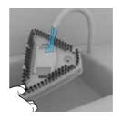
Remove any dirt /debris from the brushes and wash under running water (max  $40^{\circ}$ C). Leave to dry before re-fitting the compact scrub brush onto the steamer.
