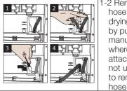
1-2 Remove the hose behind the drying machine by pulling it manually from where it is attached. Do not use a tool to remove the hose.
