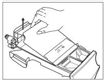
To remove any detergent residue or if you place a wrong additives in the tanks, empty the drawer in a basin or in suitable containers to collect the liquid.
