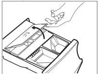
3. Gently pour only liquid detergent in the AutoDose detergent tank . Fill up to the maximum indicated level MAX
