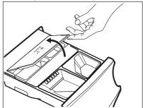
Gently pour only liquid detergent in the AutoDose detergent tank Fill up to the maximum indicated level MAX
