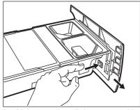
Make sure that all detergent residue is removed from the upper and lower part of the recess. Use a small brush to clean the recess.
