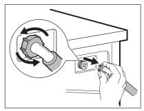
Clean the valve filter on the back of the appliance with a toothbrush.
